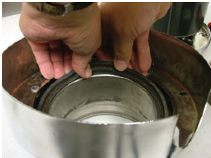
Figure 11. Replacing Shredder Gasket
