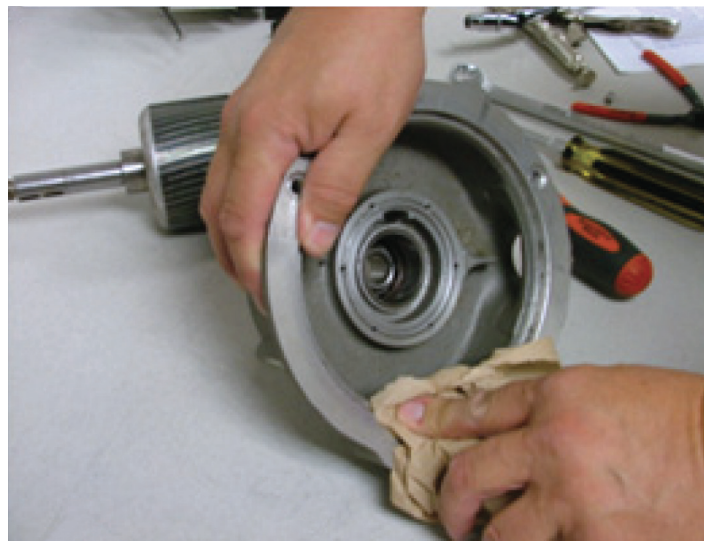
Figure 21. Cleaning Upper End Bell
